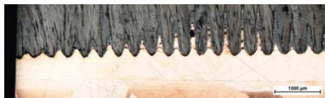
Fig. 5. Small de-bonding of outer edge after 6000 cycles IR detected before. The length of de-bonding is 5 mm. The scale represents 1000 \mu\text{m} .
